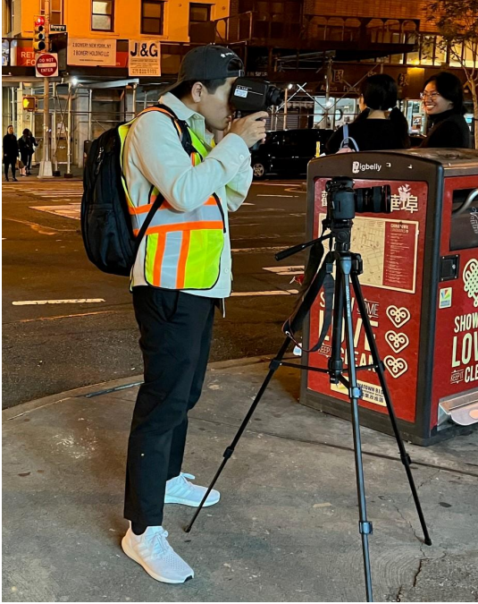
DSLR Camera, Tripod + Luminance Meter (Measure and mapping of perceived "brightness" in visual field)
