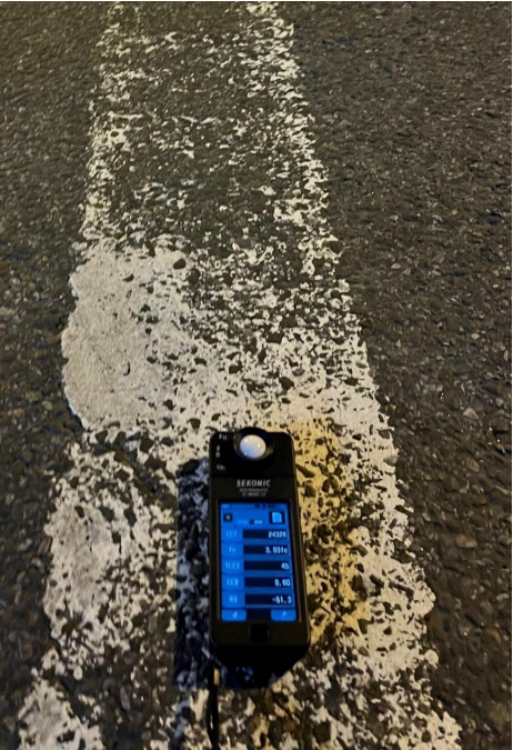
Illuminance Meter (Measure quantity of light on the ground)
