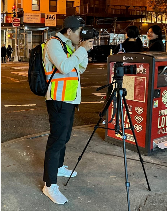
DSLR Camera, Tripod + Luminance Meter (Measure and mapping of perceived "brightness" in visual field)
